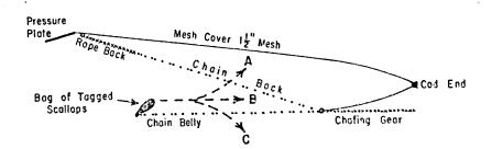
Diagrammatic vertical section through covered offshore dredge showing method of release of tagged scallops and Fig. 2. possible escape routes:
