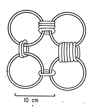
Fig. 4. Canadian offshore scallop dredge ring linkage with 1-6 links per ring.
