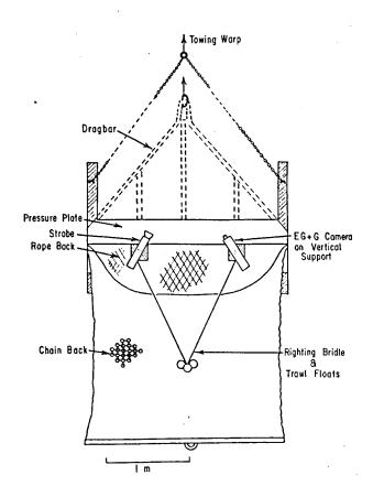
Canadian offshore dredge showing modifications for use with EG & G Camera. (Shaded areas: additions to dredge; dashed outlines: deletions). Fig. 1.
